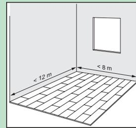
6 With room lengths of more than 12 m and widths of more than 8 m an intermediate expansion joint should be fitted. Expansion and contraction are linear so the greater the surface the larger the expansion joint needs to be. An expansion joint must be used in typical doorways and room angles. Parquet floors are not suitable for use in damp areas like bathrooms and saunas.
