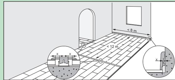
7 Before starting carefully measure the length and the width of the room to plan a precise lay-out to achieve a balanced appearance of the floor. This will ensure also you won't end up with the last row being too narrow. If the last row would be less than 40 mm the installation will be easier if you cut down the planks of the first row in the width.
